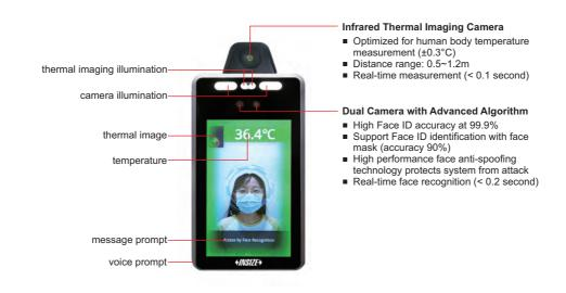
This device introduces a highly advanced built-in facial recognition algorithm and high resolution infrared thermal imaging camera. This brand new technology will identify someone by face, even while wearing a face mask. It locates the forehead and measures forehead temperature without touch. This device is the ideal solution for fully automatic contactless access control, time attendance, and temperature measurement.
