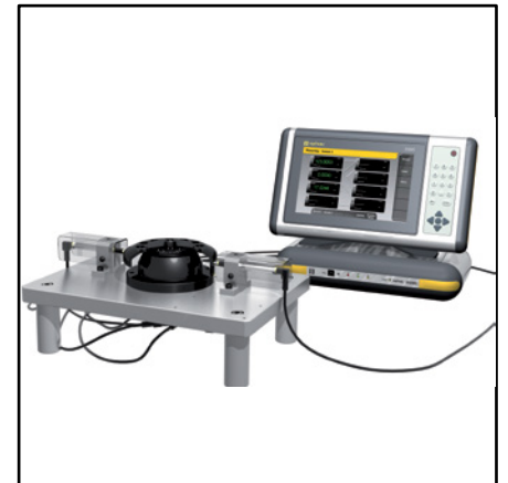
Capacitive probes on a jig
