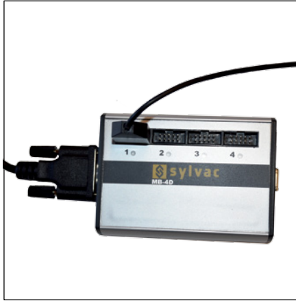
Digimatic instruments connected to a MB-4D
