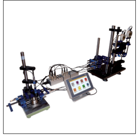
Probes and indicators connection through M-BUS inputs
