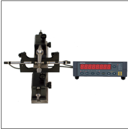
Measuring a shaft with 2 probes (A+B)
