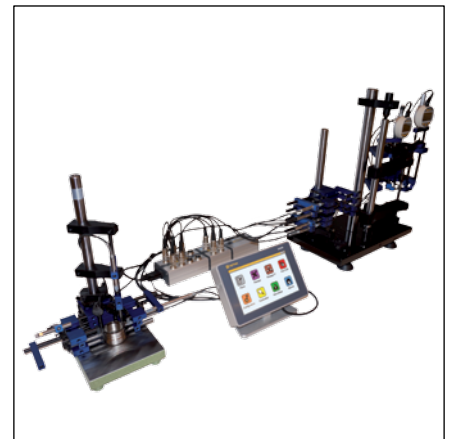
Probes and indicators connection through M-BUS inputs
