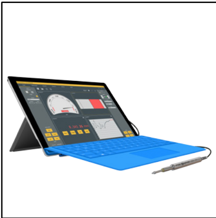
Absolute digital probes connected to a PC, measures displayed by Sylcom.
