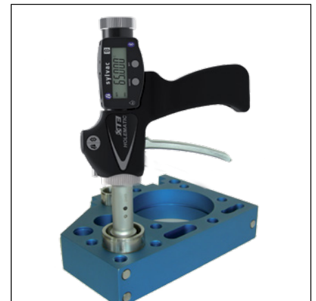
Measuring with pistol XTH system
