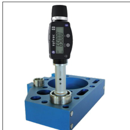
Measuring with ratchet XTD system
