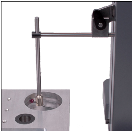
Internal groove measurement with accessories 930.2108, 930.2110 and 905.2207
