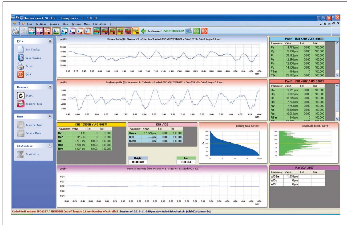
measuring software (optional), can control the roughness tester, display roughness values, profile and curve, data statistics
