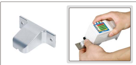
probe cover (included), can put the small workpieces directly on the probe for measurement
