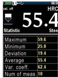
Statistics display mode, show maximum, minimum, deviation, average, relative range and test times
