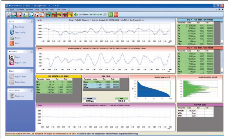
measuring software (optional), can control the roughness tester, display roughness values, profile and curve, data statistics
